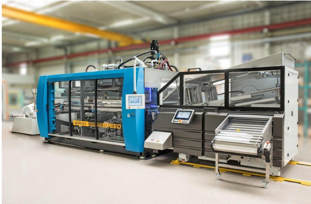
**Image: Cup Forming Machine Thermorunner KTR 5.1 Speed with PUS Stacker**
