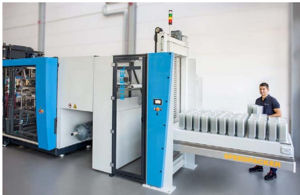
**Figure: SpeedPacker - Buffer and Unloading Station for KMD Speedformer Series**
