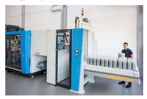
Figure: SpeedPacker - Buffer and Unloading Station for KMD Speedformer Series
