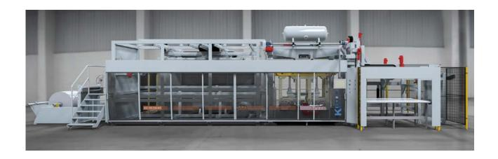
BU: Thermoforming machine KID 100/230 BFS-R with forming and trimming tool, for refrigerator liners
