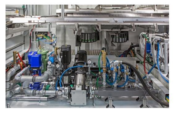
Figure 2: Two pumps and mixer valves supply the two circuits with cooling water for the upper and lower tool.
