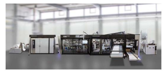
Figure 3: The new generation of cupforming machines SPEEDFORMER KTR 5.2 Speed
