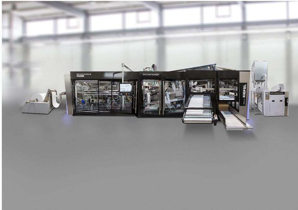
*The cup-forming KTR 5.2 SPEED machine offers increased production and maximum efficiency. © KIEFEL GmbH*
